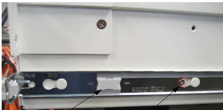
Figure 7: Optional screw hole for additional support.
