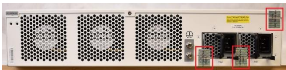
Figure 16: FG-1800F & 1801F Seal Placement
