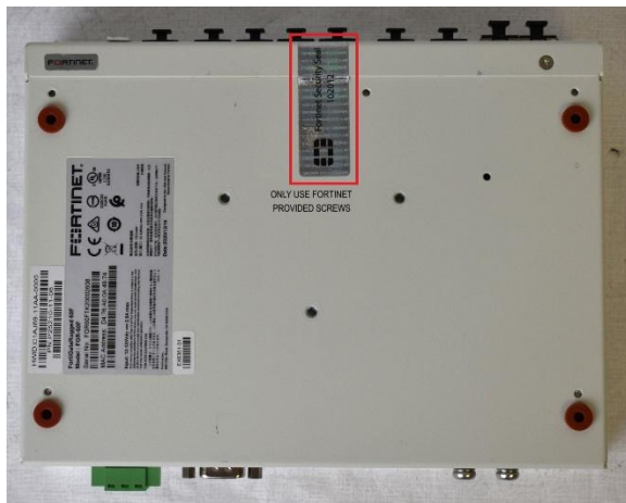
Figure 12: FGR-60F Seal Placement
