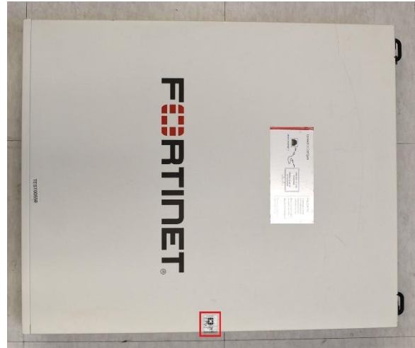
Figure 19: FG-3501F & 3501F Seal Placement
