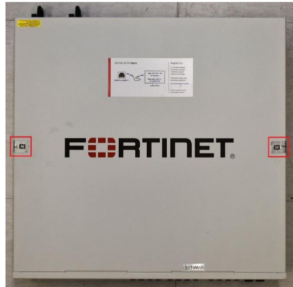
Figure 15: FG-1000F & 1001F Seal Placement
