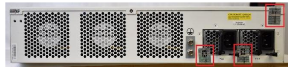
Figure 17: FG-2600F & 2601F Seal Placement
