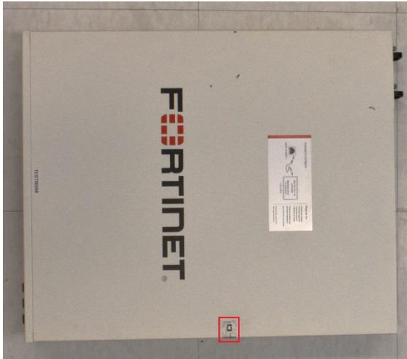
Figure 18: FG-3000F & 3001F Seal Placement
